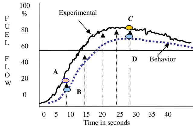
Fig.7. Closed loop behavior and experimental responses to obtain optimum PID parameters.
