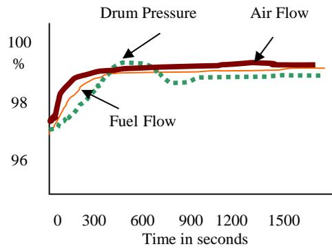
Fig.4.Open Loop ( $\Delta$  fuel flow from 95% to 100%)
