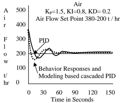
Fig.13 Air flow response for 110 to 42 MW change in load
