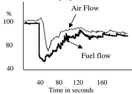
Fig. 6. Sudden run back of load due to auxiliary failure
