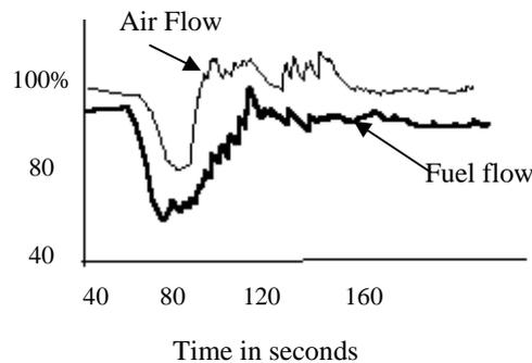
Fig. 5. Sudden load change due to grid disturbance
