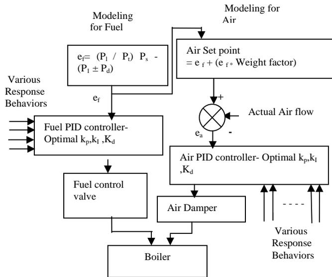
Fig.8. Modeling Based Cascaded PID Control for Fuel and Air
