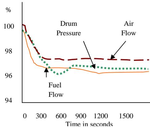
Fig.3.Open Loop ( $\Delta$  fuel flow 100% to 95%)
