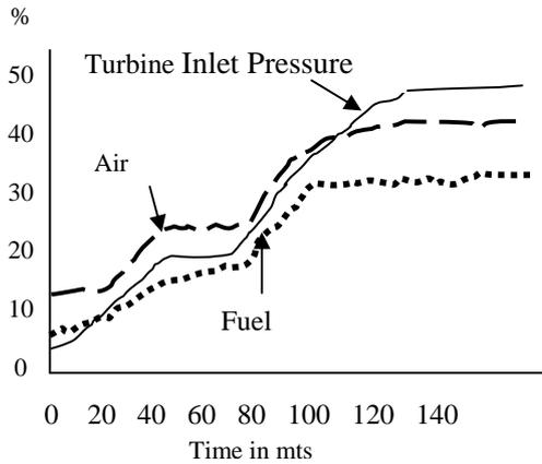
Fig.1. Boiler Start-Up curve
