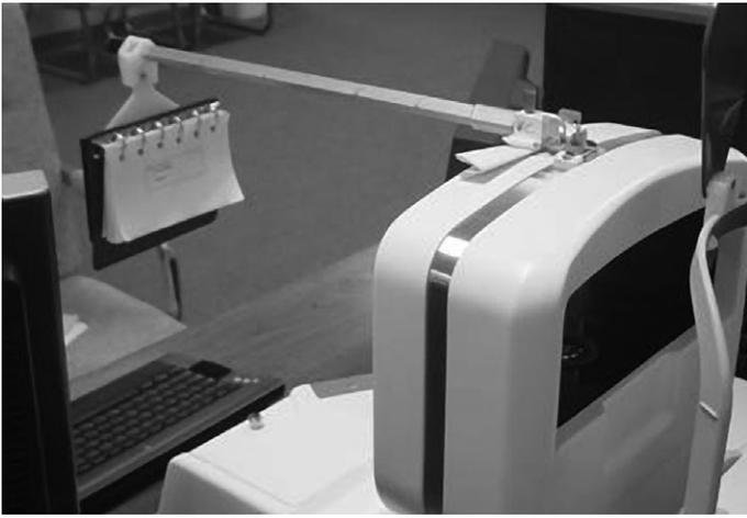
**Figure 3:** Setup for reading text with pull-down pages on the open-field autorefractor.
